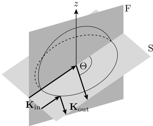
FIG. 1: The Fresnel plane (F) is spanned by the  $z$ -axis and the incident wave vector  $\mathbf{K}_{\text{in}}$  while the scattering plane (S) is spanned by the incident wave vector and the wave vector  $\mathbf{K}_{\text{out}}$  of the reflected wave. The scattering angle is denoted by  $\Theta$ .
