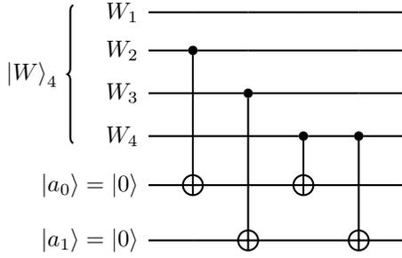
Fig. 4: Quantum circuit for generating the leader-aware state  $|\Lambda\rangle_6$  by considering the example in Figure 3. The input state of the circuit is  $|W\rangle_4 \otimes |00\rangle$ , with  $|W_i\rangle$  denoting the  $i$ -th qubit of the  $|W\rangle_4$  state. Accordingly  $|\Lambda\rangle_6 = \frac{1}{\sqrt{4}}[|10000\rangle + |010010\rangle + |001001\rangle + |000111\rangle]_{W_1, W_2, W_3, W_4, a_0, a_1}$ .
