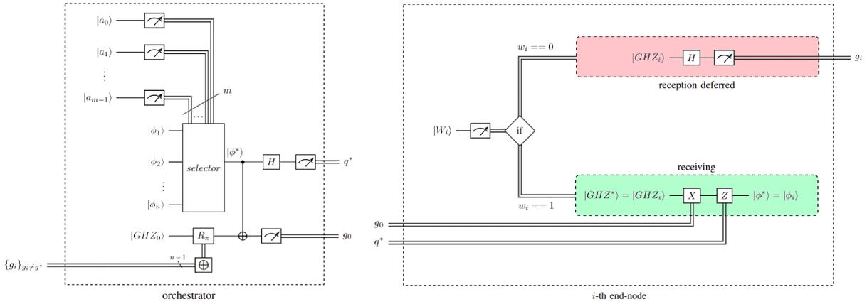
Fig. 6: Quantum circuit for downlink entanglement access.
