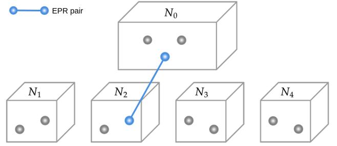
(b) Final state: contention resolution completed. An EPR between the orchestrator  $N_0$  and end-node  $N_2$  has been generated, with the orchestrator (end-node) acting as transmitter during downlink (uplink) time-slots.
