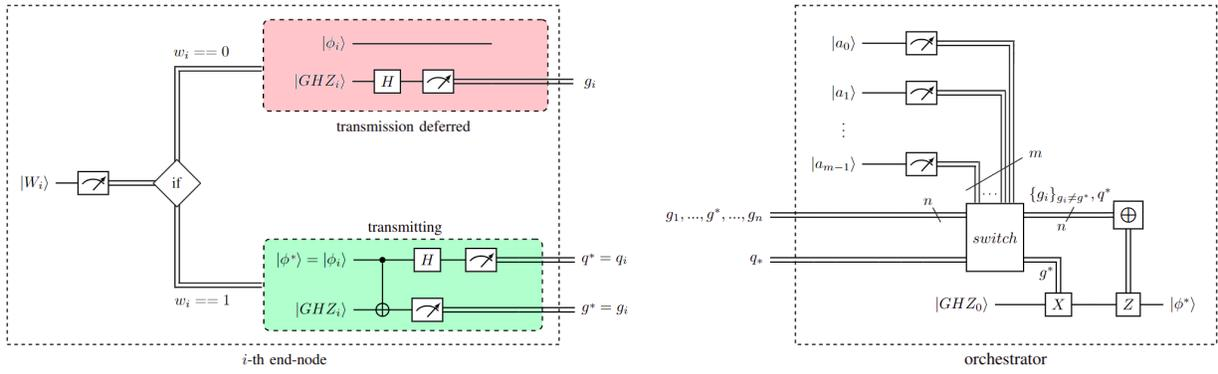
Fig. 5: Quantum circuit for uplink entanglement access.
