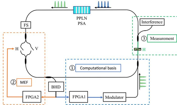
FIG. 1. Setup design of a classical implementation of Shor’s algorithm. PPLN, periodically poled lithium niobate; FS, fiber stretcher; PSA, phase sensitive amplification; BHD, balanced homodyne detector; FPGA, field programmable gate array; Modulator, a module contains the phase modulator and the intensity modulator.
