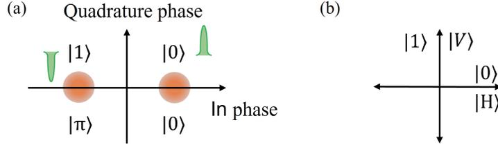
FIG. 2. Information encoded by the state of a DOPO. (a) Representation of a classical bit in the control register with the phase state of a DOPO. (b) Representation of a classical bit in the work register with the polarization state of a DOPO.
