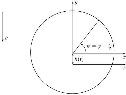
Figure 1: Inverted pendulum with a vibrating pivot point.
