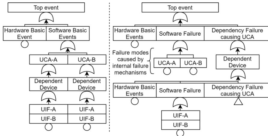
Figure 4. Left side, potential logical organization of fault tree. Right side, proposed configuration of fault tree
