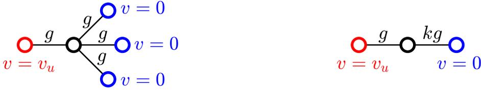
Fig. 2.2: Left: Cell with upstream and downstream neighbors at fixed voltage. Right: Downstream neighbors collapsed into a single cell.
