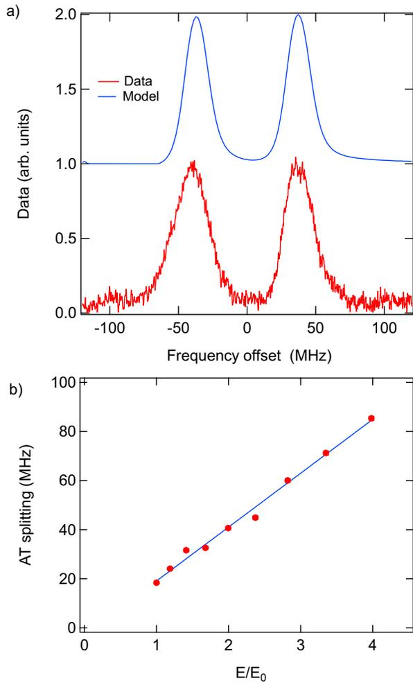
FIG. 2. (a) AT EIT Spectrum of the  $55F \rightarrow 55G$  transition with an applied rf field of 473 MHz. A simulated spectrum is offset above the data for clarity. (b) Autler-Townes splitting of the  $60F \rightarrow 60G$  EIT signal as a function of applied UHF electric field. This plot confirms the expected linear scaling between rf electric field and Autler-Townes splitting. Uncertainties are smaller than the point markers.  $E_0 \approx 0.63$  V/m.
