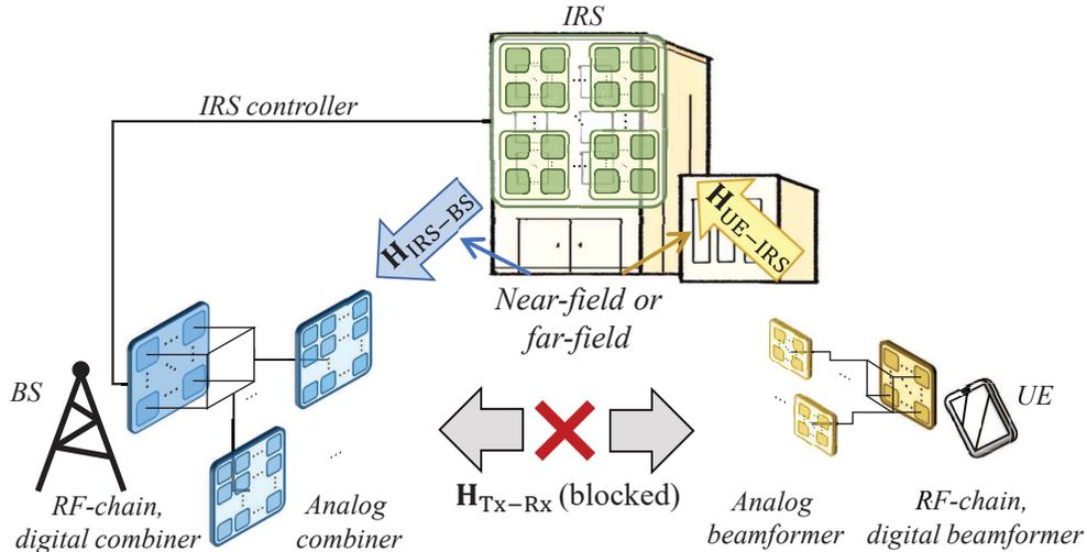
Fig. 1. Integrated THz UM-MIMO and IRS system.
