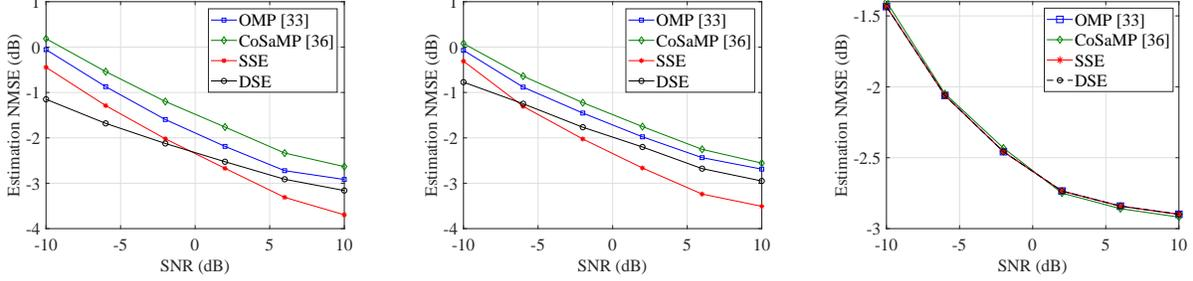
(a) WSMS system using HSPM.  $N_u = 16, M = N_b = 1024, K_u = 1, K_m = 16, M = N_b = 1024, K_u = 1, K_m = N_u = 16, M = N_b = 256, K_u = K_m = K_b = 4, T_u = 12, T_i = 768, T_b = 192$     (b) WSMS system using SWM,  $N_u = 16, M = N_b = 1024, K_u = 1, K_m = N_u = 16, M = N_b = 256, K_u = K_m = K_b = 4, T_u = 12, T_i = 192, T_b = 192$     (c) Compact array systems using PWM,  $K_b = 1, T_u = 12, T_i = 192, T_b = 192$
