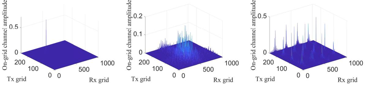
(a) Amplitude of the on-grid channel in the compact array using the DFT codebook. (b) Amplitude of the on-grid channel in the WSMS using the DFT codebook, the subarray spacing is  $64\lambda$ . (c) Amplitude of the on-grid channel in the WSMS using the subarray-based codebook, the subarray spacing is  $64\lambda$ .
