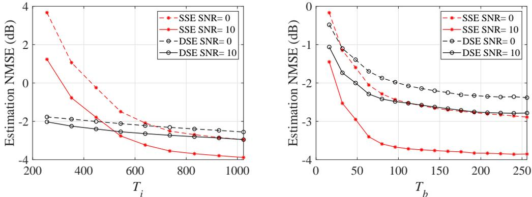
(a) NMSE against  $T_i$ ,  $N_u = 16$ ,  $M = N_b = 1024$ ,  $K_u = 1$ ,  $K_m = K_b = 4$ ,  $T_u = 16$ ,  $T_b = 192$  (b) NMSE against  $T_b$ ,  $N_u = 16$ ,  $M = N_b = 1024$ ,  $K_u = 1$ ,  $K_b = K_m = 4$ ,  $T_u = 16$ ,  $T_b = 192$ .
