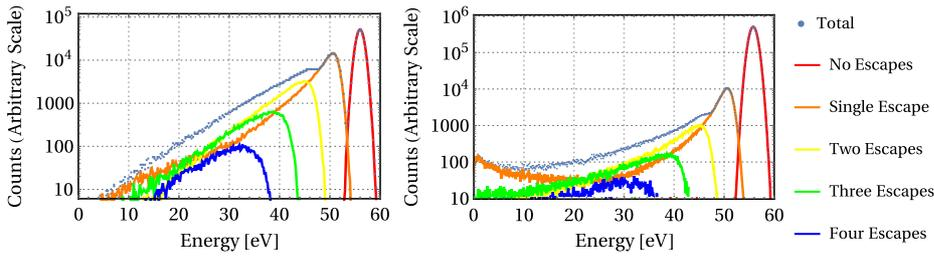
**Fig. 3** Impulse response to a 56 eV Auger electron from a fixed 10 nm implantation depth (left) and from an initial depth distribution derived from the SRIM simulation in Figure 2 (right), broadened to match the detector resolution (color online). Note the deviation from an EMG tail shape caused by 2+ electron escape, particularly at  $\sim 10$  eV below the primary peak.
