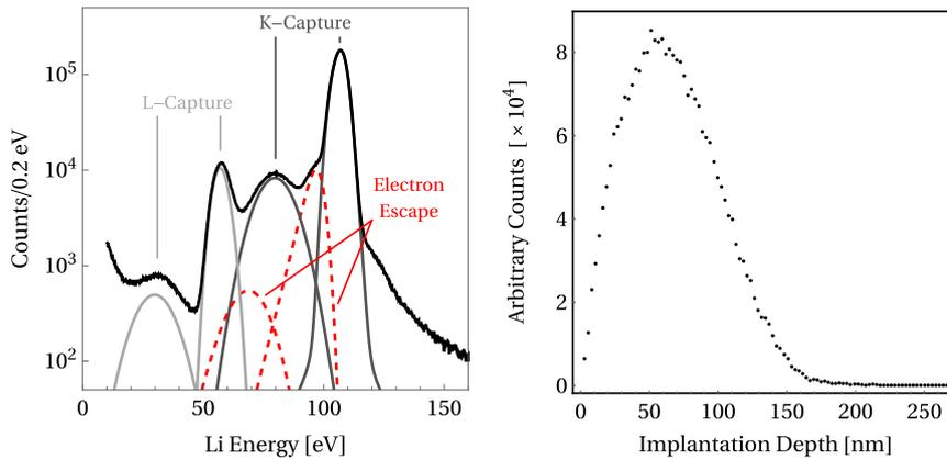
**Fig. 1** The measured  ${}^7\text{Li}$  recoil spectrum (black) shows four peaks for the different  ${}^7\text{Be}$  decay channels. Fits to the four decay channels and to the observed electron escape tails from the K-Capture peaks are shown (color online). Other fit features not shown. Figure adapted from [1]
