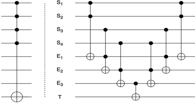
Figure 2: **Equivalent quantum circuit for four-control-one-target ( $C^4(X_5)$ ) Toffoli gate.** The four-control-one-target Toffoli gate is fed with 3 extra qubits, which act as a buffer when the Four-control-one-target Toffoli gate is decomposed into two-control-one-target Toffoli gates. It is to be observed that the extra qubits undergo two NOT gates in total, hence they will always show  $|0\rangle$  as output.
