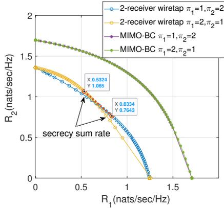
Fig. 2: Secrecy rate regions for  $K = 2$ . It is seen that encoding is determining.
