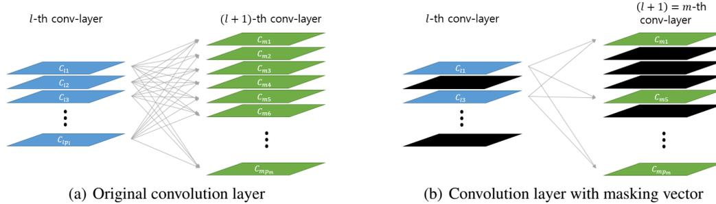
Figure 2: **Convolution layer and masked convolution layer.** Masking vector  $\mathbf{m}^{(l)}$  screens channels of the  $l$ -th layer. When  $(\mathbf{m}^{(l)})_j = 0$ , the  $j$ -th channel of the  $l$ -th layer becomes inactive. Blue and green rectangles represent input and output channels, and black rectangles represent masked channels.
