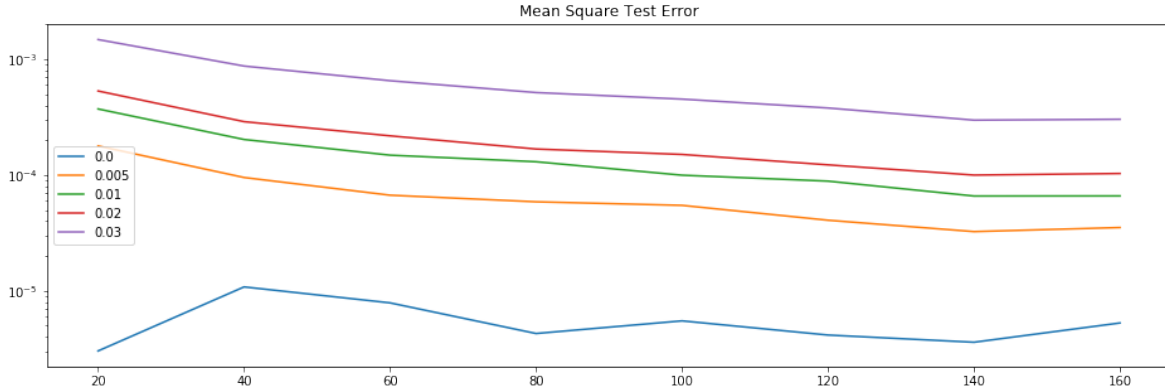
Figure 1: Mean squared errors of the approximation of the solution operator for the transmissivity identification problem on the test set for five different noise levels: 0.00, 0.005, 0.01, 0.02, 0.03. The x -axis shows the ambient dimension which corresponds to the number of measurements D , the y -axis records the mean squared error of the reconstruction over the test set.
