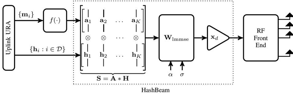
Fig. 2. This figure illustrates the downlink beamforming process employed by HashBeam. The uplink URA scheme provides channel estimates and hashes for the uplink message associated with each decoded user. The Khatri-Rao product of the hashes and the channels is computed, and downlink beamforming vectors are computed via uplink-downlink duality. The sum of all beamforming vectors is then transmitted by the base station.
