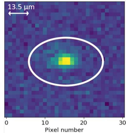
Fig. 2. Ion picture obtained from the average of  $\sim 4000$  sequences after a 1 s dark time when the ion has been voluntarily warmed up at the end of the cooling period. The counts number is indicated by the color scale. The red elliptical contour represents the area outside of which the baseline plane is fitted and inside of which data are fitted.
