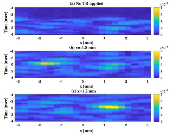
Figure 4. The TR spatiotemporal focusing capability of the subTHz system in Fig. 1(c) operating at 273.6 GHz with bandwidth  $B = 3$  GHz for different Rx positions. The received signal strength without applying TR is also sketched.
