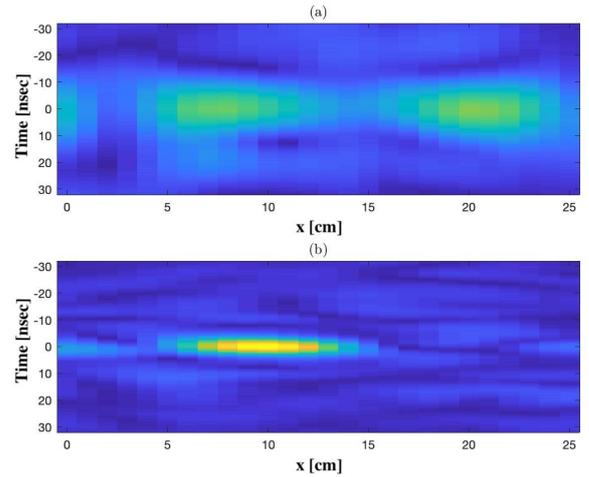
Figure 2. Measurements for the TR spatiotemporal focusing capability of the  $8 \times 1$  MISO wireless system at different Rx positions and different bandwidth values  $B$ : (a) two Rx positions at  $x = 7.5$  cm and  $x = 20$  cm with  $B = 100$  MHz; and (b) the Rx is positioned at  $x = 10$  cm and  $B = 400$  MHz.
