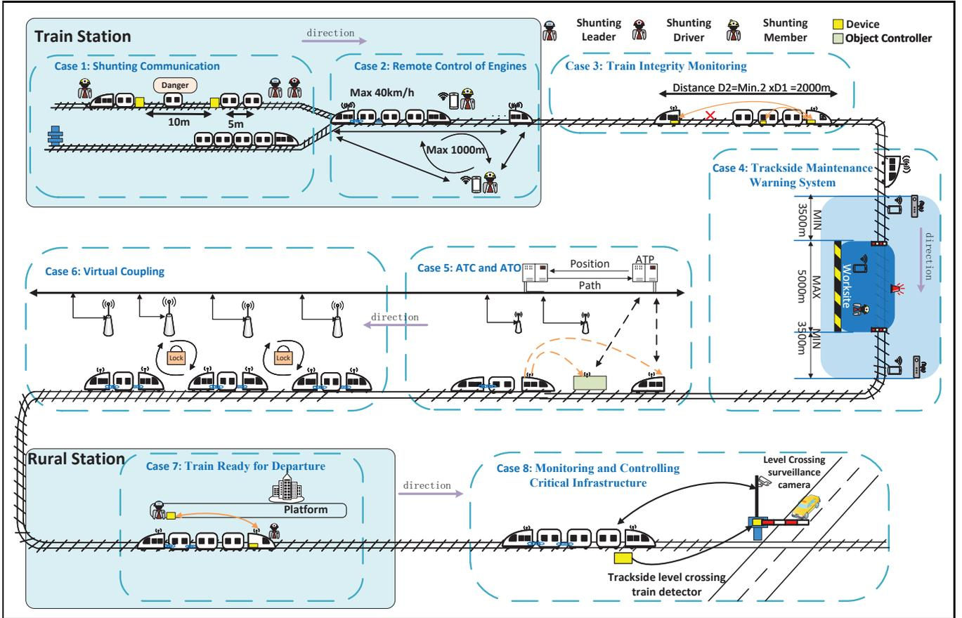
Fig. 1. Use cases of off-network communication in FRMCS.
