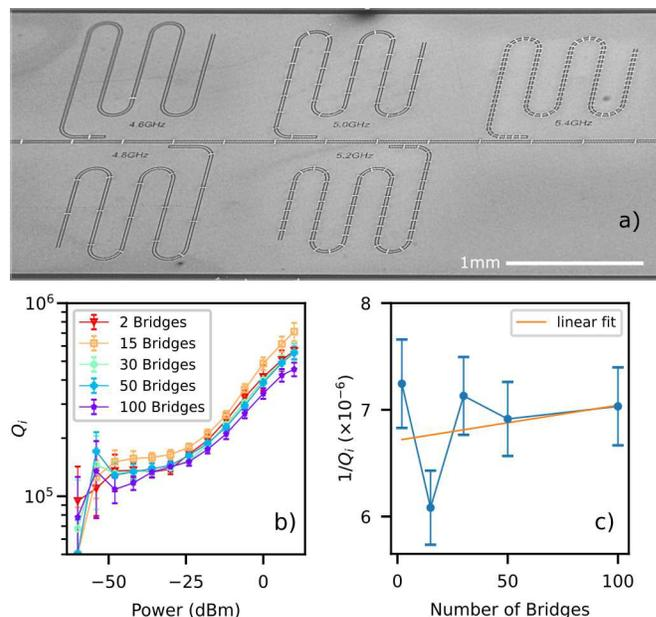
FIG. 3. a) SEM picture with a tilted angle of a device formed of five resonators coupled to a common feedline. b) Quality factor versus microwave power for each resonator (dots, with lines as guide to the eye). The number of bridges fabricated on the resonators range from 2 to 100. c) Loss (inverse quality factor) versus number of bridges at  $-30 \text{ dBm}$  where the system enters the desaturated limit (dots) and a linear fit (continuous line).
