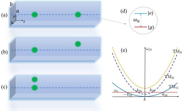
FIG. 1. Schematic illustration of two atoms couple to the waveguide with a  $a \times b$  rectangle cross section. (a) The two atoms are both located in the middle axis of the waveguide. (b) One of the atom is off-centered. (c) The connection between the two atoms is perpendicular to the axis of the waveguide. (d) The energy-level diagram of the atoms. (e) The energy spectrum of the waveguide.
