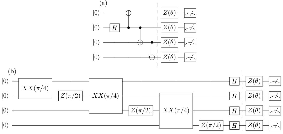
FIG. 6. Four-qubit circuit decomposition used for the GHZ magnetometry problem for (a) IBM and (b) ion-trap architectures.
