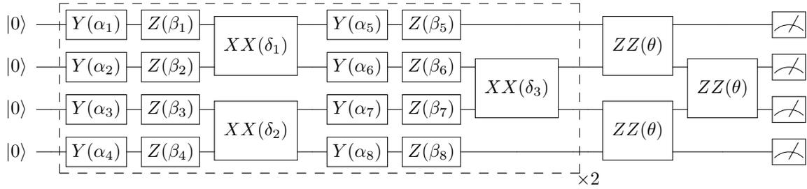
FIG. 8. Four-qubit circuit decomposition used for the Random Unitary.
