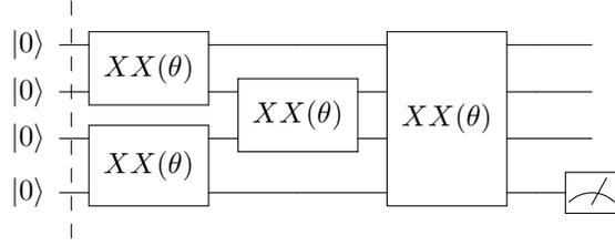
FIG. 7. Four-qubit circuit decomposition used for the spin squeezed state setup.
