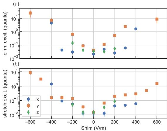
FIG. 3. The sensitivity of the c. m. and stretch mode axial excitation to changes in the bias electric field along the  $\hat{x}$  (blue circles),  $\hat{y}$  (orange squares), and  $\hat{z}$  (green diamonds) directions.
