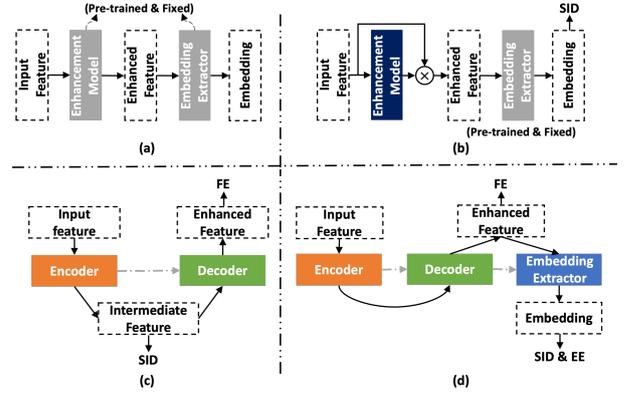
Figure 1: Block diagrams of noisy speech compensation approaches for speaker verification tasks. (a): Pretrained enhancement model, (b): VoiceID loss [11] ( $\otimes$  denote element-wise multiplication), (c): U-Net-based system (Proposal 1), (d): Extended U-Net (Proposal 2)
