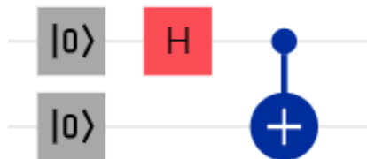
Figure 3. After the CNOT gate on the right, an entangled state is formed: \frac{1}{\sqrt{2}}(|0\rangle|0\rangle + |1\rangle|1\rangle) .
