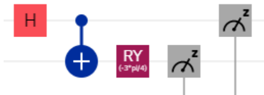
Figure 6. Circuit to determine \langle A_1 B_2 \rangle , with \alpha_1 = 0 and \beta_2 = 3\pi/4 .
