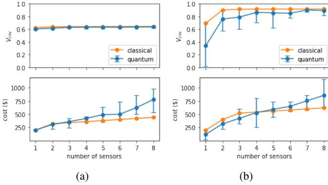
Fig. 3: Comparison of coverage and cost of selected sensor configurations obtained from the classical and quantum solutions for the left side (discretized into  $4 \times 4$  grids) of the vehicle, when (a) the orientation of the sensors was fixed perpendicular to the surface, (b) the sensors could be oriented at four different angles.
