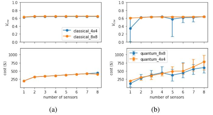
Fig. 4: Comparison of coverage and cost for  $4 \times 4$  and  $8 \times 8$  discretization on the left side, with all sensors oriented perpendicularly outwards to the surface, for (a) classical and (b) quantum method.
