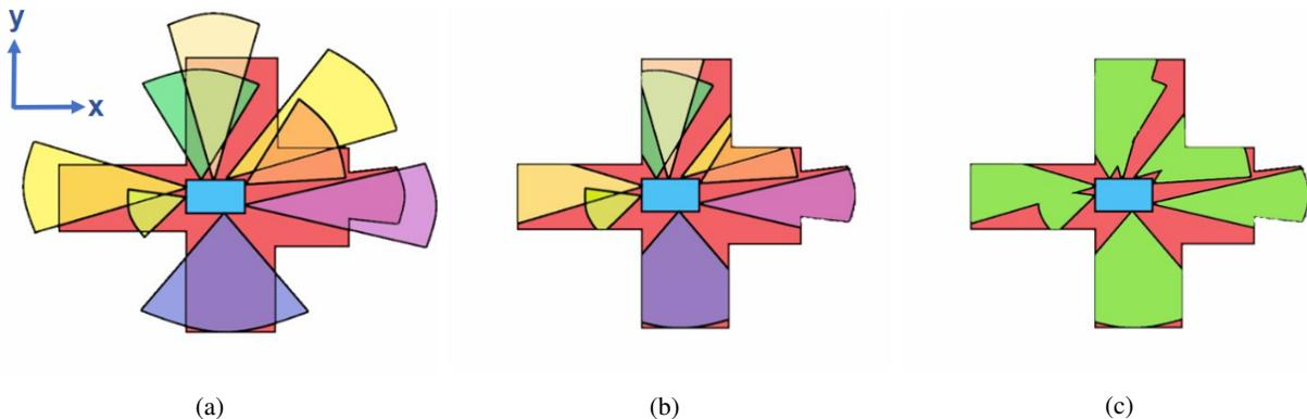
Fig. 1: Figure (a) depicts the FoVs of individual sensors placed at different positions of the vehicle (blue rectangle, with *front* towards the positive  $x$ -direction) at different orientations using various colours. Only the portions of the FoVs that lie within the red RoI adds to the coverage, as shown in (b). The effective-FoV (green) and coverage provided by the sensors is portrayed in (c).
