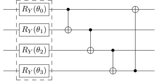
Fig. 2: First layer of the Basic Entangling Layers ansatz acting on 4 qubits. The parametrized rotation gates are followed by multiple *CNOT* gates, the target qubit of each gate is determined using the relation  $t = (c + l + 1) \bmod n$ , where  $c$  and  $t$  are the control and target qubit numbers,  $l$  is the ansatz-layer being constructed and  $n$  is the number of qubits the ansatz operates on. An  $L$ -layer ansatz avails  $nL$  optimizable parameters.
