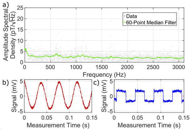
FIG. 4. **Rabi magnetometry.** (a) Amplitude spectral density of a 1-second measurement with no signal field applied. The units are calibrated by the slope and the NV gyromagnetic ratio as discussed in the main text. (b) Measurement of a separate  $\delta B_{\text{MW}} = 4.4$  nT, 25-Hz amplitude modulated magnetic field with 100% modulation depth. (c) Measurement of a separate  $\delta B_{\text{MW}} = 2.2$  nT, 25-Hz phase modulated magnetic field with a  $\pi/4$  phase deviation.
