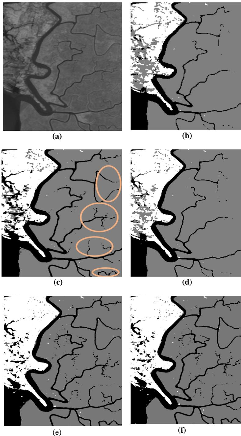
**Figure 1:** (a) Original image. Blue, Red, Green, NIR, SWIR-1 and 2 bands are used in the study. NIR band is presented here. (b) detection of classes from original image (c) detection of classes from 3 times upsampled image (SRCNN) (d) detection of classes from 3 times upsampled image (bicubic interpolation) (e) detection of classes from
