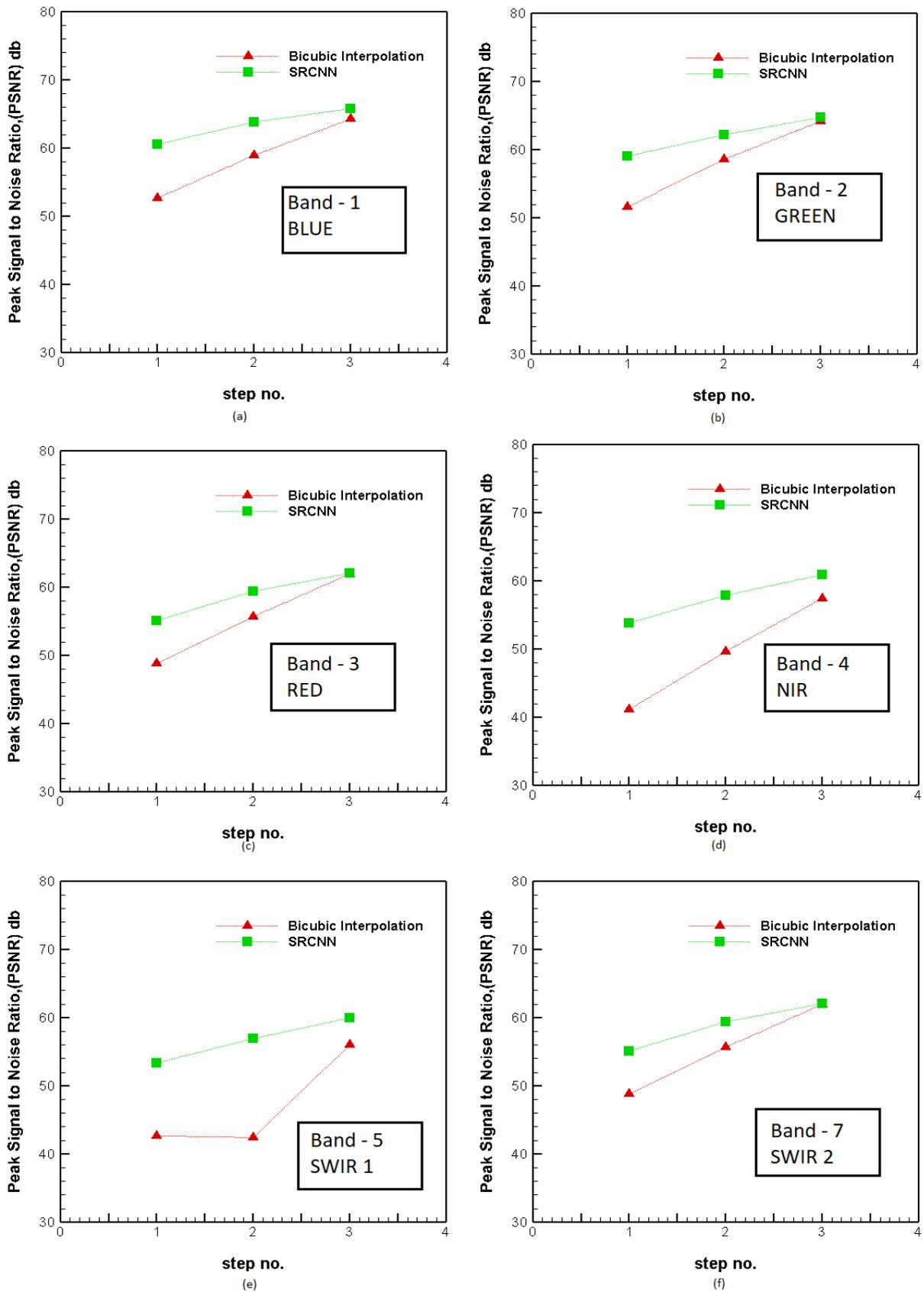
Fig 2. Variation of Peak Signal to Noise Ratio for LANDSAT 7 ETM+ Bands 1-6 and 7 with the change of degree of image upscaling for SRCNN and Bicubic interpolation method. Any nth step corresponds to a 3 times up-sampling
