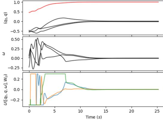
Figure 7: An example trajectory for the TRACE system using the actor network as the controller. The value of  $q_0$  is in red and  $q, \omega$  in black. Note that the control inputs resemble that of a smoothed, bang-bang controller which one expects to observe for minimum time solutions.
