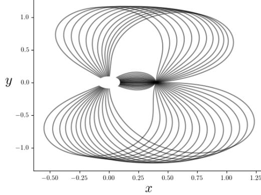
Figure 6: Actor feedback control over sample trajectories in the  $(x, y)$  space near the target. Each trajectory begins with an initial heading  $\theta(0) \in [-\pi, \pi)$ . There is a paradigm switch between trajectories facing near the target to begin to face about 45 degrees away, corresponding to a kink in the value function. The choice of steering left or right when facing exactly opposite to the target also corresponds to a kink.
