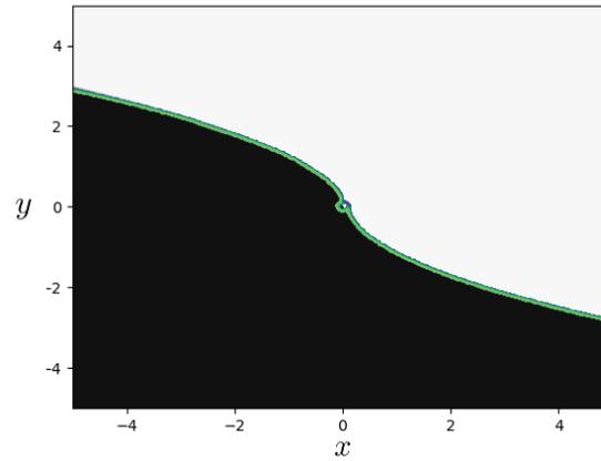
Figure 1: Switching surface given by neural network actor with tanh activation (white/black) and switching curve computed by grid-based semi-lagrangian iteration (green)
