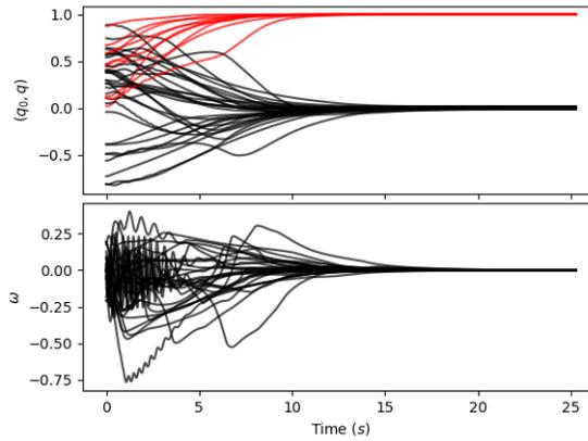
Figure 8: Ensemble trajectories displaying stability of the neural network controller.
