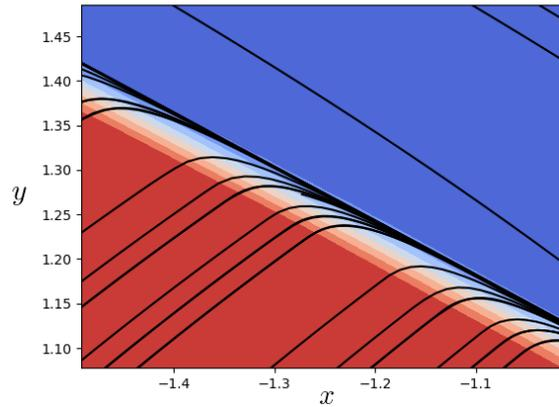
Figure 2: Close up of switching curve given by neural network actor with sample trajectories overlaid (black).
