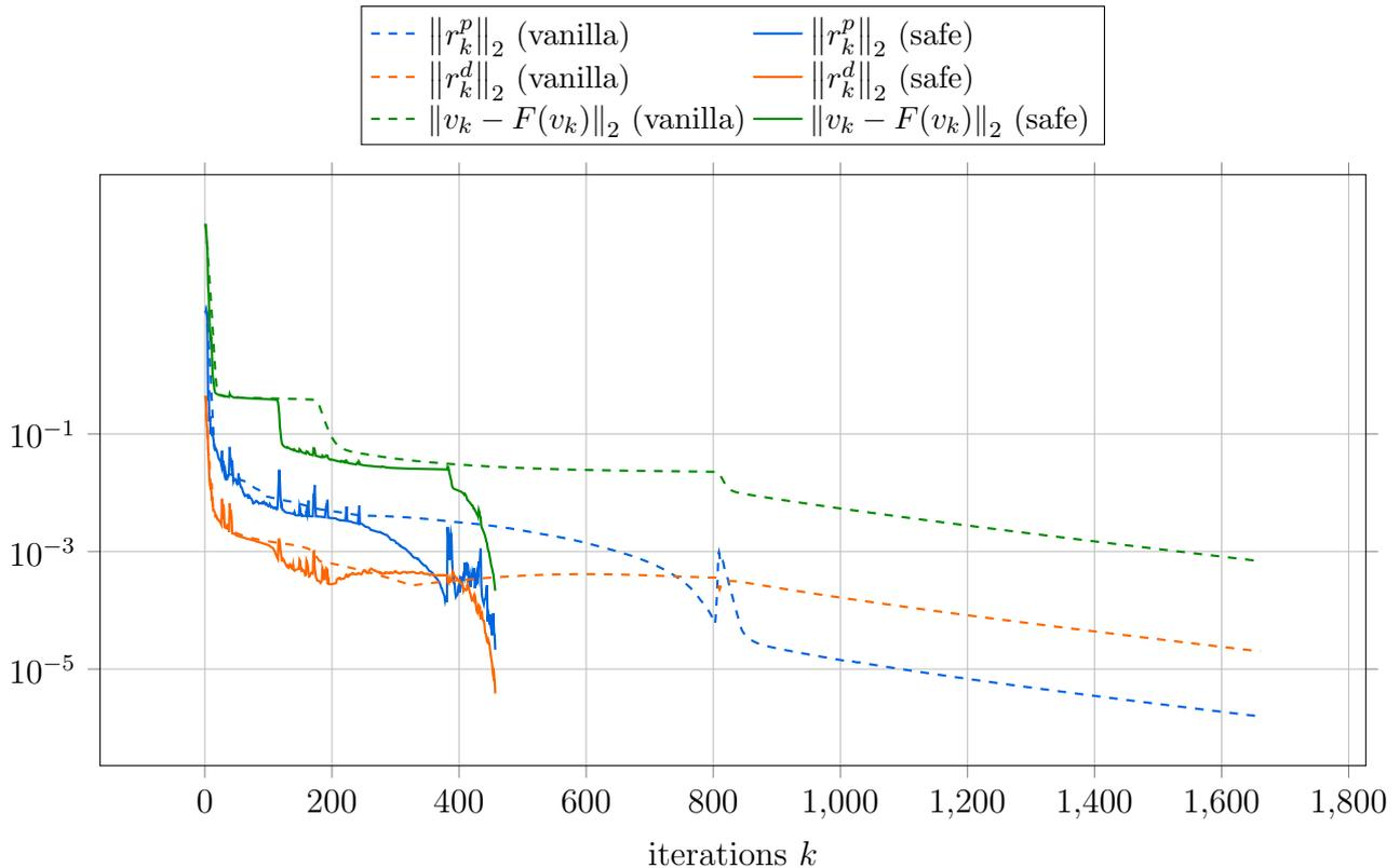
**Figure 1:** Norms of primal residual  $\|r_p^k\|_2$ , dual residual  $\|r_d^k\|_2$ , and fixed point residual  $\|v_k - F_p(v_k)\|_2$  of the vanilla and the safeguarded accelerated method (Mittelmann: `ros_500`).
