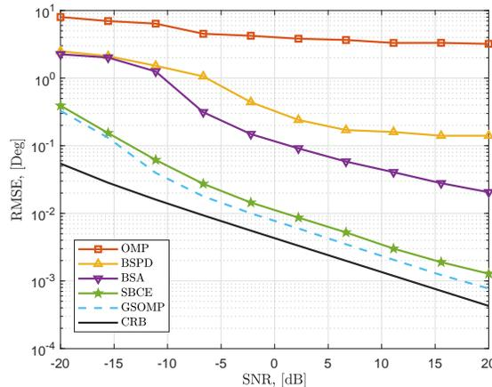
Fig. 3. Physical channel direction RMSE versus SNR.
