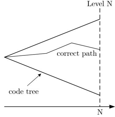
Fig. 3. Decoding tree of PAC codes.
