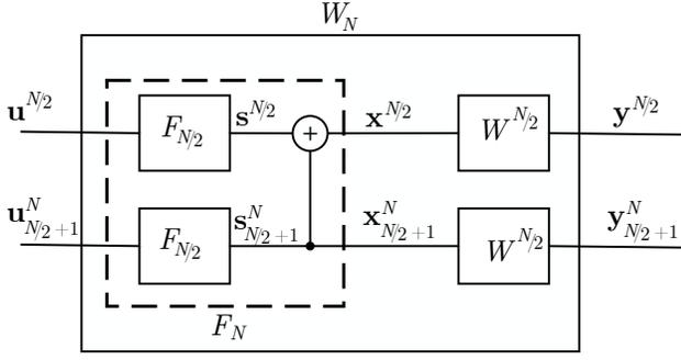
Fig. 4. Recursive construction of polar code of length  $N$ .
