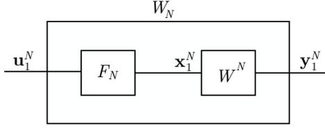
Fig. 2. Polar code construction of length  $N$ .
