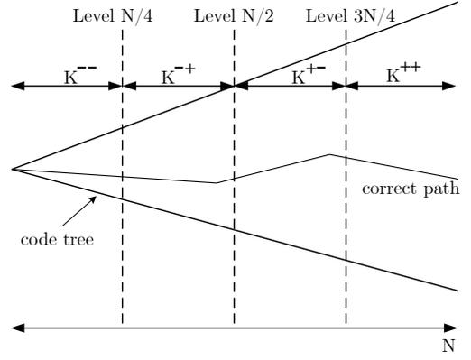
Fig. 6. Decoding tree of PAC codes after two step polarization.
