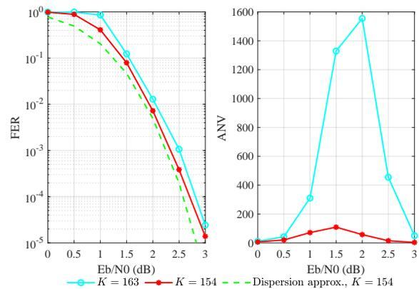
Fig. 16. Performance comparison of the PAC codes of length  $N = 256$  with different data lengths.
