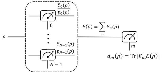
FIG. 1. Schematic diagram of the experimental scheme to obtain experimental QND fidelity. For density matrix  $\rho$ , the probability of the first measurement outputting  $m$  is  $p_m(\rho)$ , while the probability of the second measurement outputting  $m$  is  $q_m(\rho)$ , which relates to the non-selective state  $\mathcal{E}(\rho)$  after the first measurement. In our proposed method, only computational basis states are needed to be prepared to obtain the QND fidelity.
