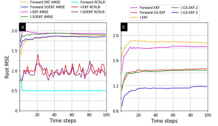
Fig. 1. AMSE and RCRLB for forward and inverse filters: (a) SOEKF; (b) GS-EKF (I-GS-EKF-2 and I-GS-EKF-5, respectively, for  $\bar{l} = 2$  and 5); compared to EKF and I-EKF, averaged over 500 runs.
