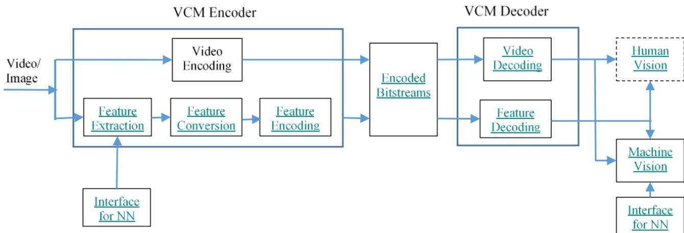
Fig. 1. The potential VCM architecture [33]
