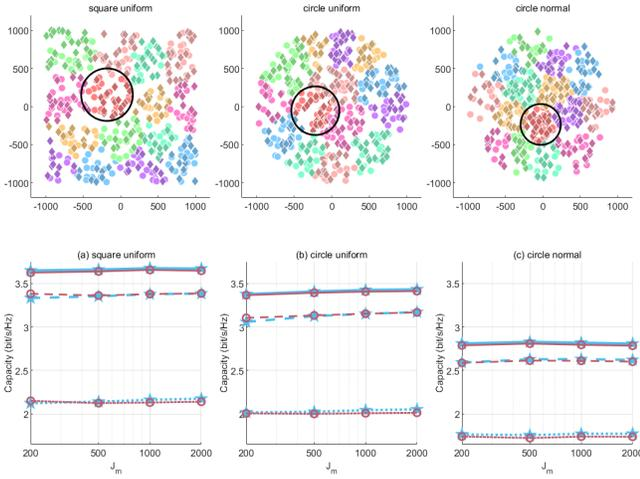
Fig. 1. Top row: illustration of  $C^2$  networks with three different settings. Different colors represent different clusters. Brighter dots represent BSs, and darker diamonds represent users. Bottom row: the capacity calculated by CDM (blue pentagram) and MPM (red circle). There are three different users-to-BSS ratios, which correspond to the dotted line  $\beta = 8$ , the dashed line  $\beta = 2$ , and the solid line  $\beta = 0.5$ , respectively.
