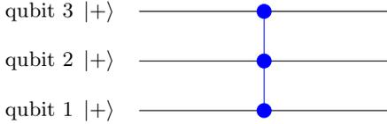
(b) Quantum circuit for generating the hypergraph state corresponding to the hypergraph given in figure 2a
