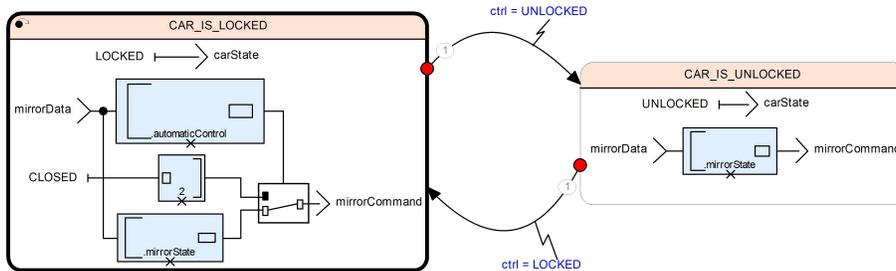
Figure 1: A sample SCADE model for a car wing mirror controller
