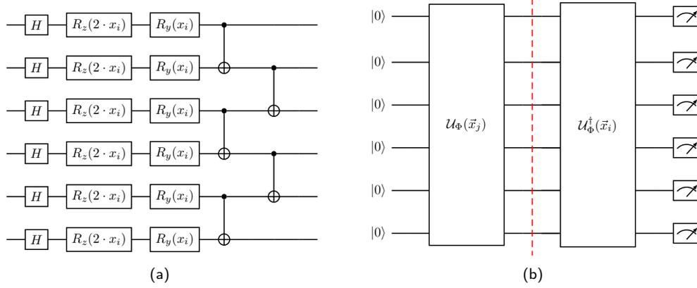
**Figure 2:** (a) Quantum circuit of the quantum feature map  $\mathcal{U}_{\Phi(\vec{x})}$  in our study. It is constituted by single-qubit rotation gates ( $H$ ,  $R_z$  and  $R_y$ ) and two-qubit CNOT entangling gates. (b) Quantum circuit for evaluating the kernel entry between two data points  $\vec{x}_i$  and  $\vec{x}_j$  in our study.
