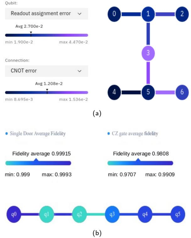
**Figure 5:** The topology structure of the (a) 7-qubits in the IBM Nairobi and (b) 6-qubits in the Origin Wuyuan quantum chip systems. For (a), our study uses qubit 0, 1, 2, 3, 4, and 5.
