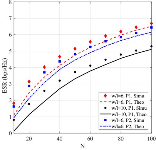
Fig. 3: Simulation and theoretical results for ESR versus the number of element  $N$  with  $b = 1$ ,  $\kappa = 5$ ,  $\sigma_j^u = 0.1$ ,  $\sigma_j^e = 0.2$ ,  $C_n^2 = 10^{-13}$ ,  $P/\delta^2 = 260$  dB.
