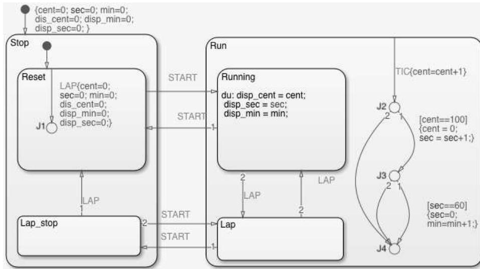
Figure 1: Simple Stateflow diagram - timer example [19].
