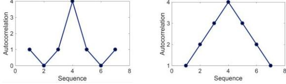
(a) Autocorrelation for the Barker code (+1, +1, +1, -1) (b) Autocorrelation for the sequence (+1, +1, +1, -1)
