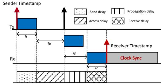
**Figure 2. Traditional clock synchronization for homogeneous devices**
