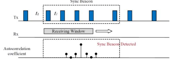
**Figure 5. 5-packets beacon detection at the ZigBee device**
