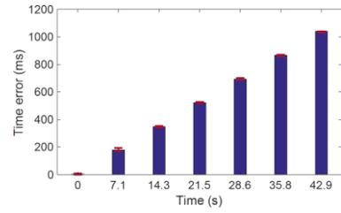
Figure 12. The time error between two devices quickly grow over time without skew calibration
