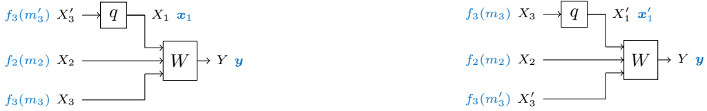
(a) X'_3 - X_1 - X_2 X_3 Y Markov chain holds approximately. (b) X_3 - X'_1 - X_2 X'_3 Y Markov chain holds approximately.
