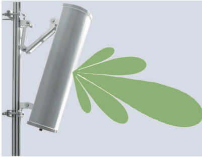
(a) Cellular BS with \theta_{tilt} \in [0, \frac{\pi}{12}]
