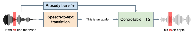
Fig. 1: Illustration of the cascade expressive S2ST framework investigated in this work. It comprises an S2T model and a controllable TTS model.
