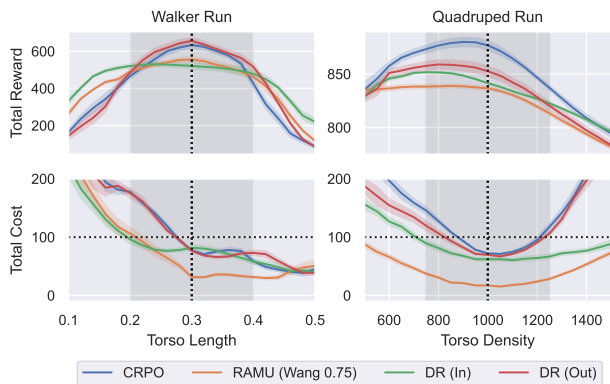
Figure 3. Comparison with domain randomization over a range of environment perturbations. Grey shaded area denotes the training range for DR (In). Shading denotes half of one standard error across policies. Vertical dotted lines represent nominal training environment. Top: Total reward. Bottom: Total cost, where horizontal dotted lines represent safety budget.
