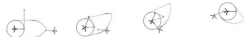
Fig. 7. Evader keeps pursuer from entering reachable set, and hence avoids collision (animation at [44]).
