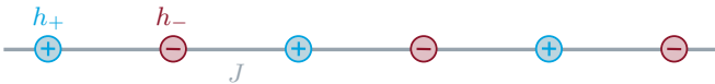
Figure 1. Transverse field Ising chain in a staggered magnetic field. The magnetic field has alternating strengths h_+ and h_- indicated by blue and red circles, respectively. Nearest-neighbor spins are coupled by an Ising interaction of strength J , marked in gray.
