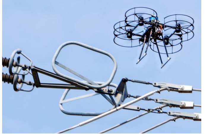
Figure 1. UAV performing visual inspection on a power transmission line.
