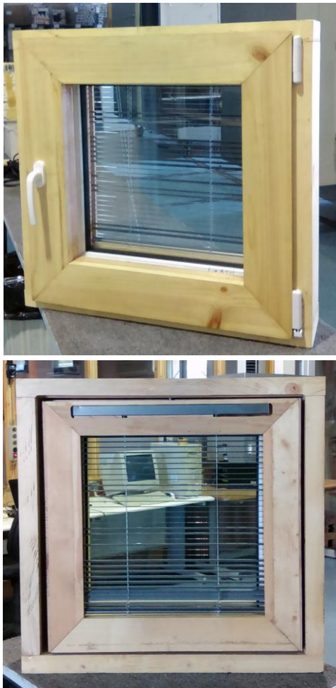
Figure 2: Mock-up model of the new daylighting system; Upper image: Casement frame, Bottom image: Pivoted window outfitted with blind
