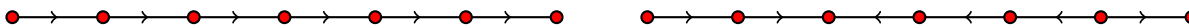
Figure 7: A no-zig-zag path (left) and a zig-zag path (right) on six vertices.
