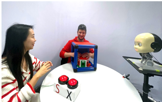
Fig. 1. Experimental setup. Two participants adopt the roles of a guide (left) and an actor (center) while the iCub robot (right) observes their gameplay. The actor inserts an object into the sorter following the guide’s instructions.
